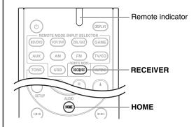
To reset the remote controller to its factory defaults, while holding down **RECEIVER**, press and hold down **HOME** until the remote indicator lights (about 3 seconds). Within 30 seconds, press **RECEIVER** again.
